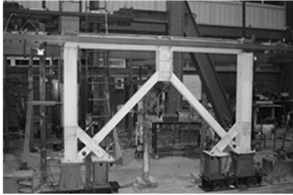
Fig. 2. Photo of the test setup and specimen with the proposed two-level control system
